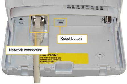
Module 1 is supplied with power via the network cable.
