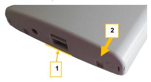
Next, remove the network cable from the network socket. Then hold down the reset button with a pointed object (bent paper clip, ballpoint pen) and plug the network cable back into the network socket.
